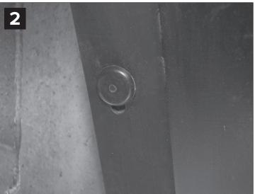
Remove original arch. Sit new arch in place. Line up holes. Fix new arch in place. Starting from centre top working your way down either side.
